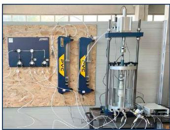
Examples of Cyclic Triaxlab installed in laboratories in Italy
