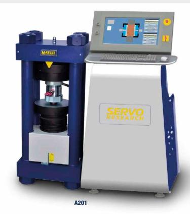
This innovative all-in-one power and control unit, specifically designed for the automatic execution of uniaxial and triaxial testing on rock cores,
