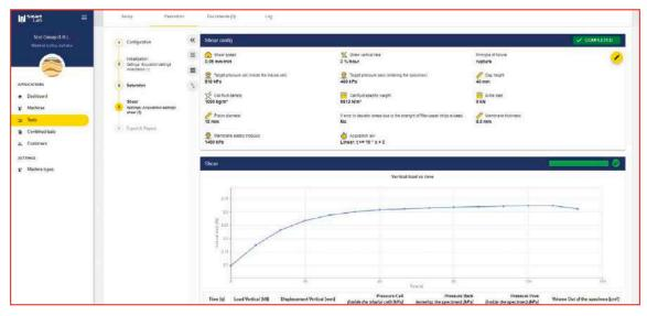
Shear phase during a triaxial test
