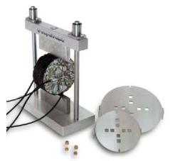
**B253-KIT** Indirect Tensile modulus, creep compliance and strength using on-specimen transducers
