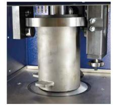
Compaction phase: simultaneous action of a static compression and of the shearing action
