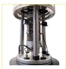
Asphalt specimen with on-specimen LVDTs and load cell
