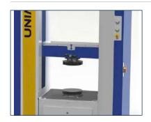
**H012-20** Platens with Ø 216 mm (details at p. 411) **SSW-LINK or C109-10N** Software for compression test (details at p. 20-21)
