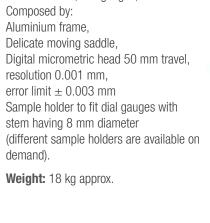
S390N CALIBRATION UNIT FOR EXTENSOMETERS AND DIAL GAUGES
