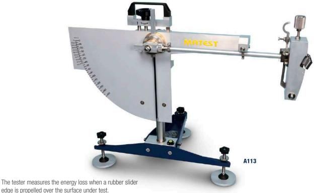
edge is propelled over the surface under test.
