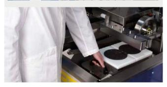
TABLE OF ACCESSORIES TO PERFORM DRY (AIR) AND WET (WATER) TEST FOLLOWING - EN 12697-22 AND AASHTO T324 SPECIFICATIONS
