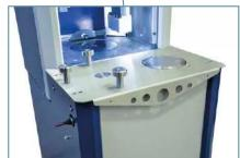
Integrated electromechanical extruder and balance
