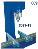
C091-13 UPPER TAMPER (steel made), for concrete KERBS tests.
