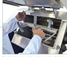
Detail of the detachable mixing shaft with helical blades
