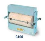
C103 SPLITTING TENSILE test device for self blocking pavers and cubes. EN 1338, 12390-6
