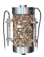
**B264-KIT** Direct tension testing kit Comprises:
