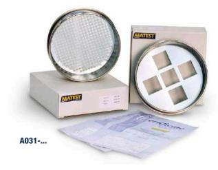
Note: EN 933-2 Standard specifies that "sieves with opening 4 mm and over shall be perforated plate square hole".
