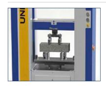
H012-21 Jig for flexural test in 3 or 4 points, rollers Ø30x160 mm
