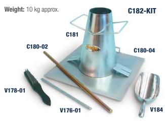
**C178-KIT** PORTABLE SLUMP CONE TEST SET, including:
