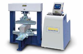
Configuration according to ASTM C1609
