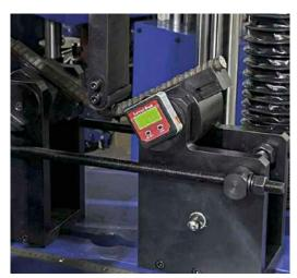
H001B-41 this jig is equipped with inclinometer
