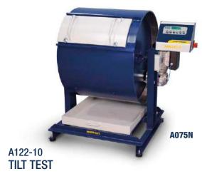
The instrument measures the roughness coefficient of a joint. The unit is also designed to test the possible fluage tendency of bituminous mixtures covering a slope of a dam subject to high sun radiations. The fluage tendency is the permanent viscous deformation of a material. The apparatus consists of an inclined adjustable plane on which the sample is placed.
