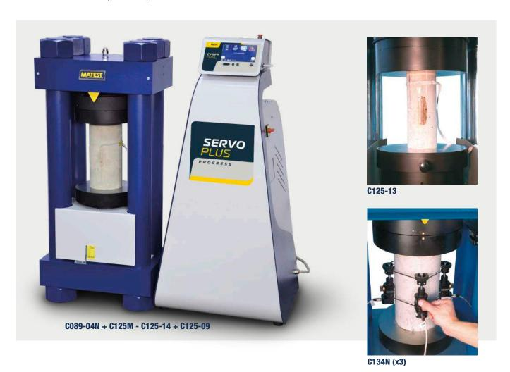
It can be used with a MATEST high stability frame 2000 or 3000 or 5000 kN capacity, coupled to the automatic servo-controlled system "Servo-Plus Progress" (mod. C104N) housed in a separate pyramidal frame.
