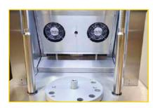
Recirculation fans ensuring uniform temperature in the chamber.
