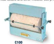
C103 SPLITTING TENSILE test device for self blocking pavers and cubes. EN 1338, 12390-6.
