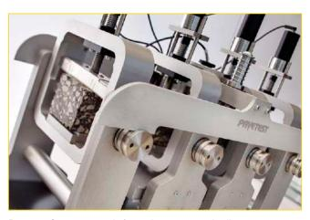
**B210-01** Servo-pneumatic four point apparatus, detail
