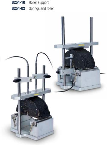
B254-02-KIT AASHTO | ASTM SCB testing kit
