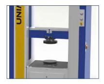
**H012-20** Platens with diameter 216 mm, complete with seatball Vertical distance between the platens: 60 ÷ 900 mm
