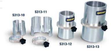
DOLLY FOR EXTRACTION, to extrude the specimen from the core cutter.
