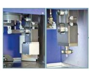
Automatic angle adjustment with double calibration AASHTO and EN or AS at 2 and 3 Automatic final flattening cycle (0°)
