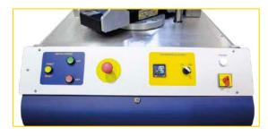
Thermoregulation display to monitor the temperature in real time.
