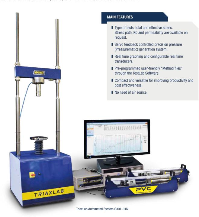
Matest TRIAXLAB is an outstanding system specifically designed for advanced soil testing.
