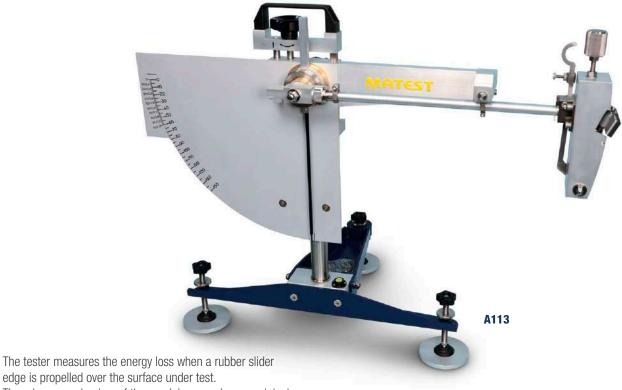
edge is propelled over the surface under test. The release mechanism of the pendulum arm has an original
