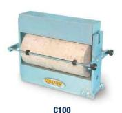
SPLITTING TENSILE test device for self blocking pavers and cubes. EN 1338, 12390-6 Technical details: see p. 289)
